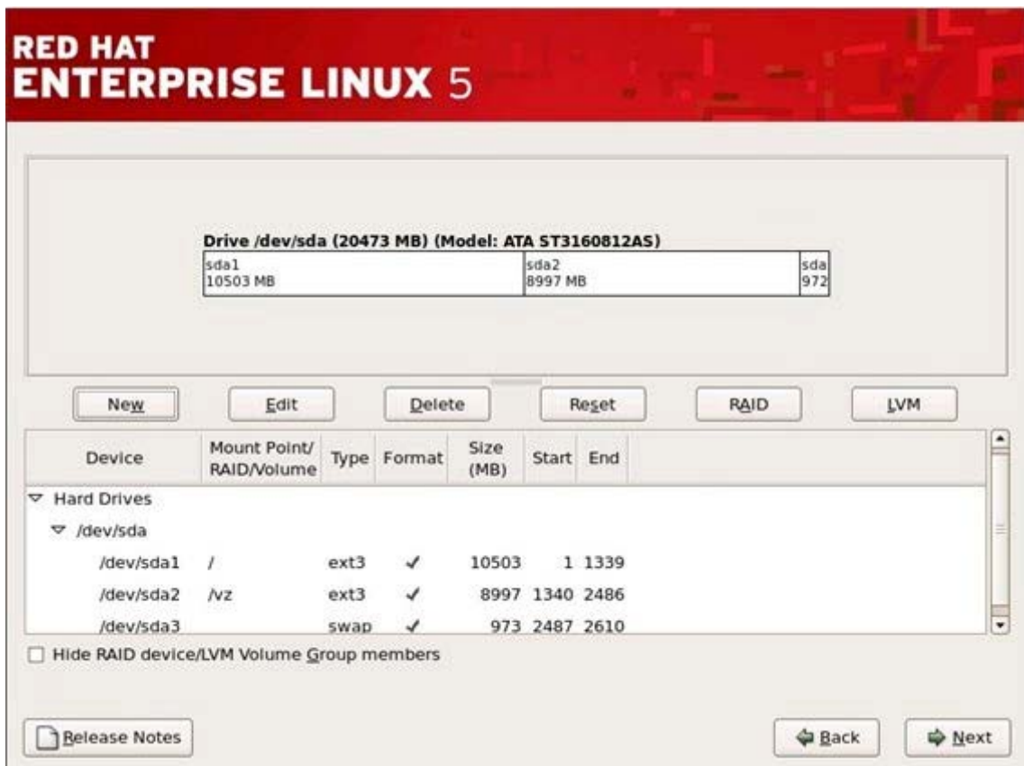
Figure 4: Red Hat Enterprise Linux Installation - Disk Druid
